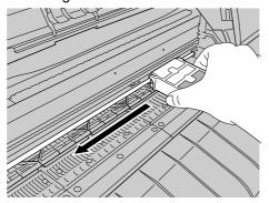
**6** With the black sponge surface on the rail, place the rail cleaner on the right side of the carriage rail, then move the rail cleaner all the way to the left end of the carriage rail.
